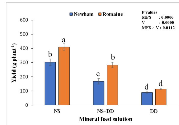
Figure 5: Effects of DD and inorganic nutrient solution on yield of two lettuce varieties tested in hydroponic system. Vertical bars are means of three replications ±SE. Bars sharing the same letter, for individual factors and interaction, do not differ significantly at LSD ≤ 0.05; NS = nutrient solution; NS+DD = 50% NS + 50% DD; DD = dairy digestate; MFS= mineral feed solution; V = varieties; MFS × V = interaction between mineral feed solution and varieties
